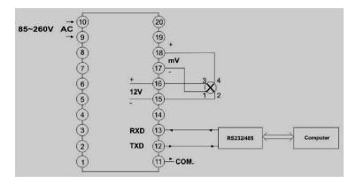
2. Used with pressure sensor. The instrument can supply DC 12V auxiliary power, and the sensor output is 2mV/V. Select input signal mV.
